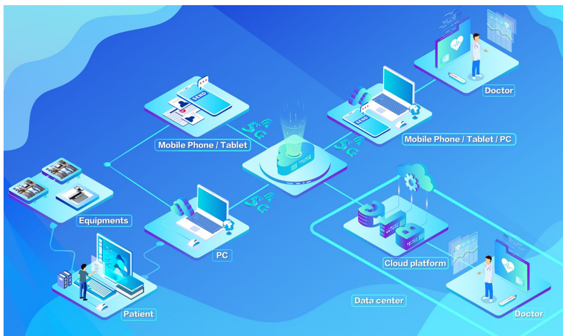
Fig. 1. Three-level linkage of the nCapp diagnosis and treatment system for COVID-19 based on the Internet of Things “cloud plus terminal”.
