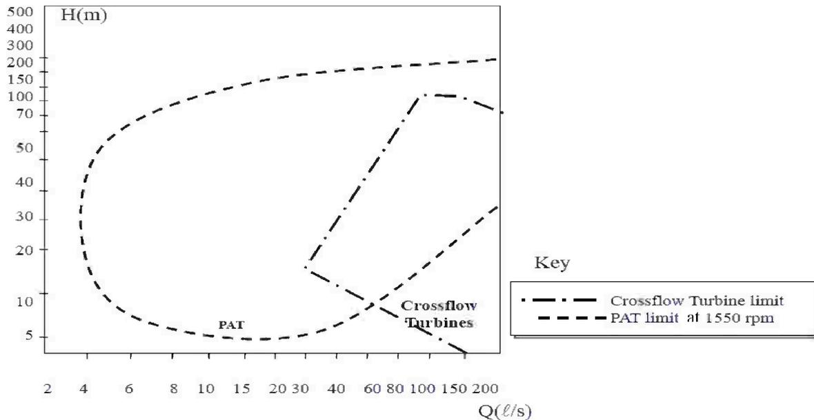
Figure (1-9) Head and flow ranges for various turbines [8]
