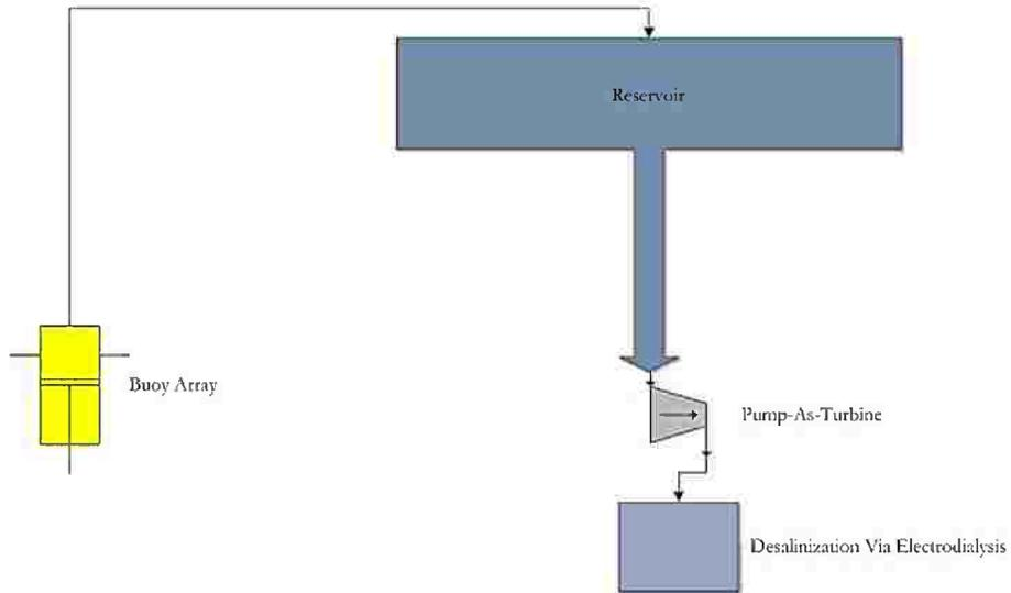
Figure (1-4) A schematic diagram of the desalination plant [3]
