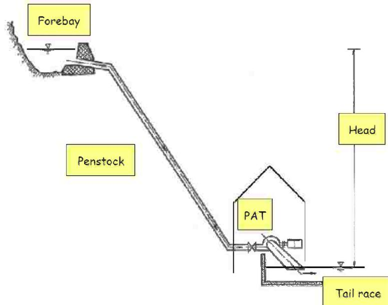
Figure (0-1) Conceptual sketch of a PAT system [1]
