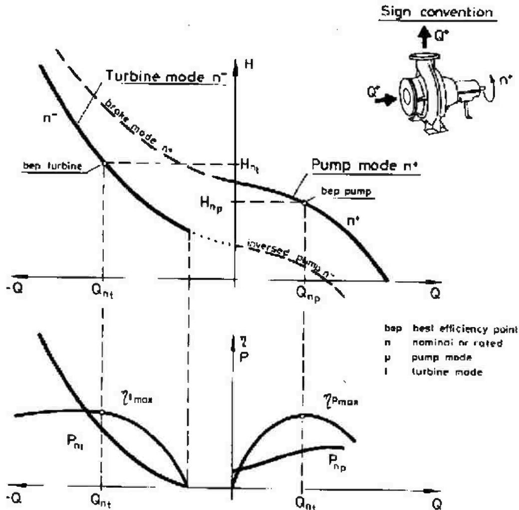
Figure (1-10) Complete characteristics of centrifugal pump for a constant speed [2]
