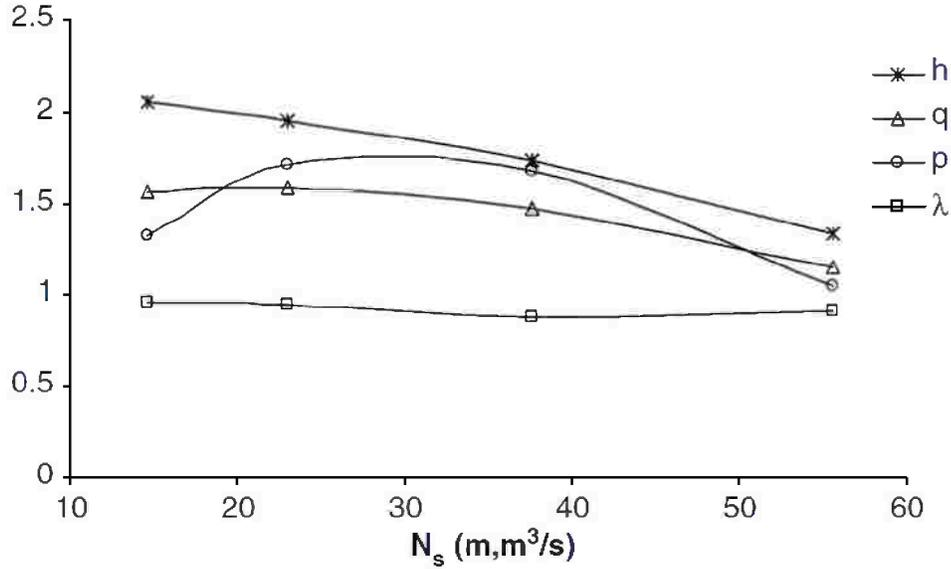
Figure (1-12) Dimensionless BEP of tested PATs [17]
