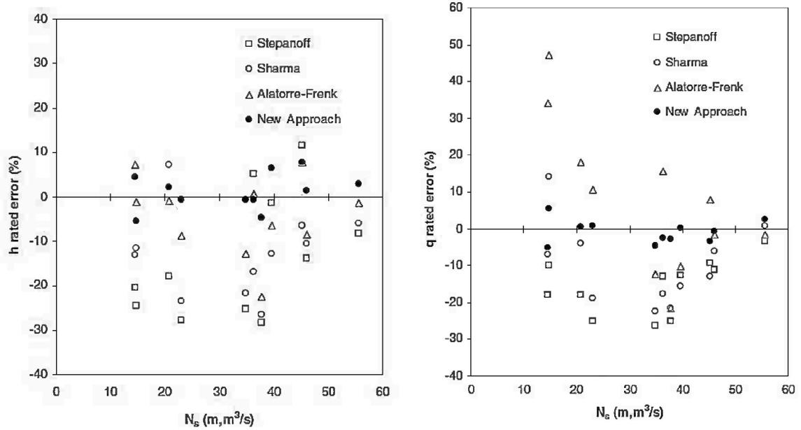
Figure (1-13) Rated errors in  $h$  and  $q$  from experiment and various methods [17]
