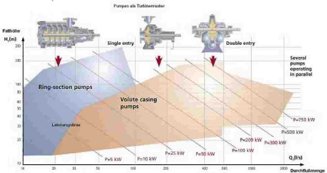
Figure (1-7) The application range for using section and volute casing pumps operating as turbines [7]
