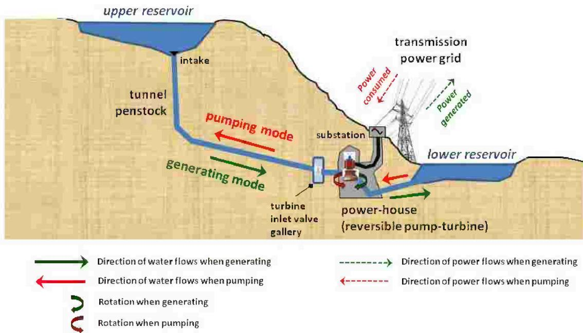
Figure (1-5) Pumped storage plant [4]
