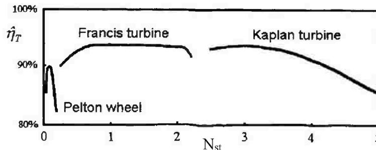
Figure (1-8) Relation between dimensionless specific speed  $N_{st}$  and  $\eta_T$  [5]
