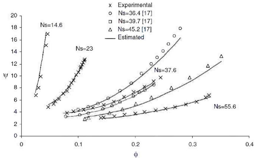
Figure (1-14) Measured and estimated PATs dimensionless head curves [17]
