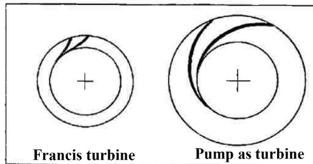
Figure (1-6) Comparison between the runner of a Francis turbine and the runner of a PAT for a similar performance based on a drawing by Meier [5]
