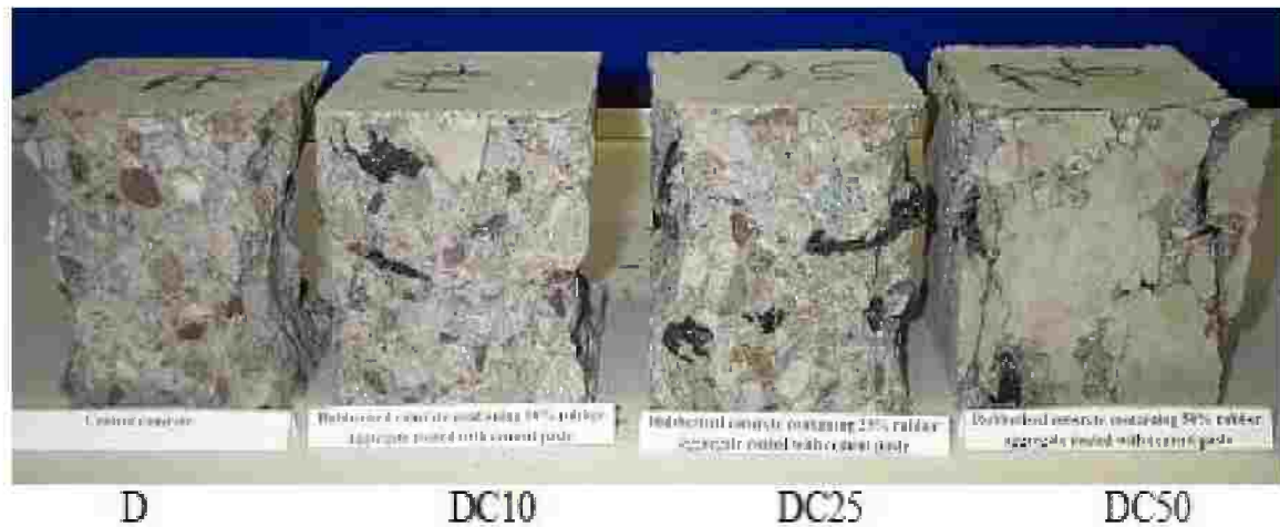
Figure 2.20 Compressive strength test samples of the rubberized concrete containing rubber particles coated with cement paste
