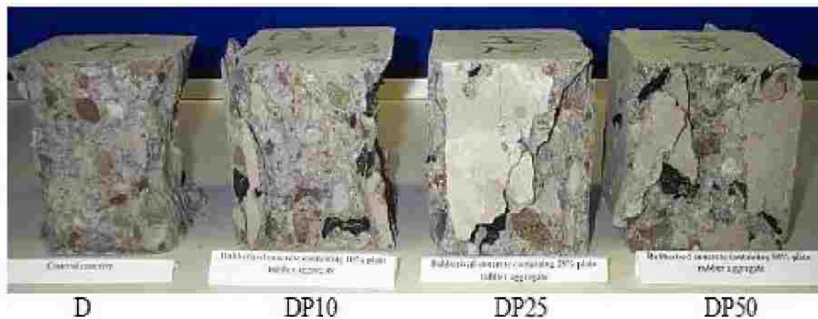
Figure 2.21 Compressive strength test samples of the rubberized concrete containing plain rubber particles
