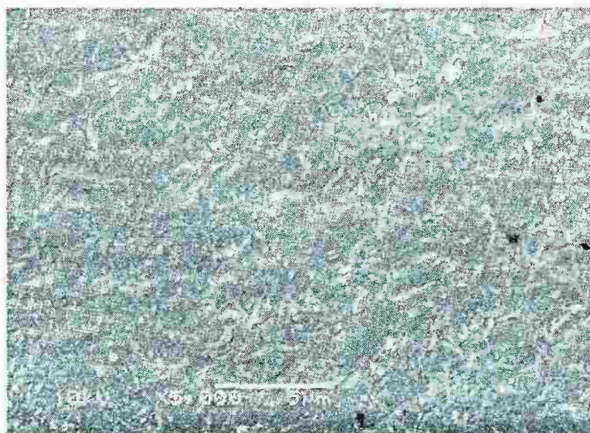
Figure 33b: SEM micrograph of PU/ SMA- ALA-MMT, 10 wt. % ( V_d )
