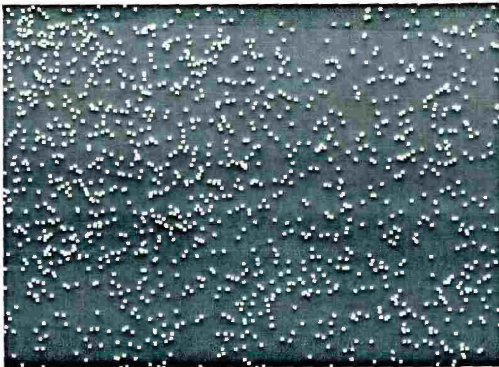
Figure 29b: Elemental mapping for Si of PU/Tyr-MMT nanocomposite 3 wt. % (III b )
