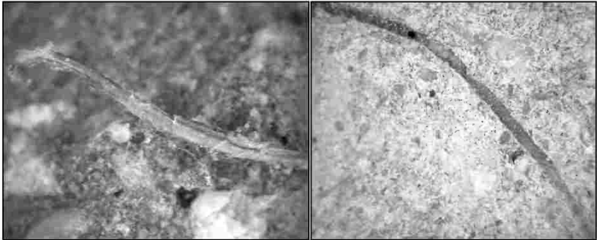
Fig. 2.47 (a) - After heating to 150°C, the fibers are still there (melting temp. \approx 150\text{-}170^\circ\text{C} ).of the fibers is left.
