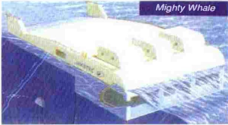
*Mighty Whale is a prototype of an offshore floating wave energy generator (Japan Marine Science and Technology Center)*
