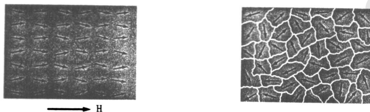
Fig. 6.11. Magnetic domains: unmagnetized and partially magnetized.
