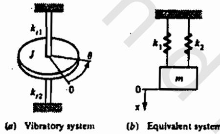
(a) Vibratory system (b) Equivalent system
