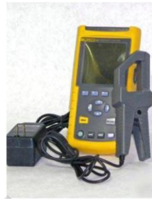
Figure 10: Power quality analyzer
