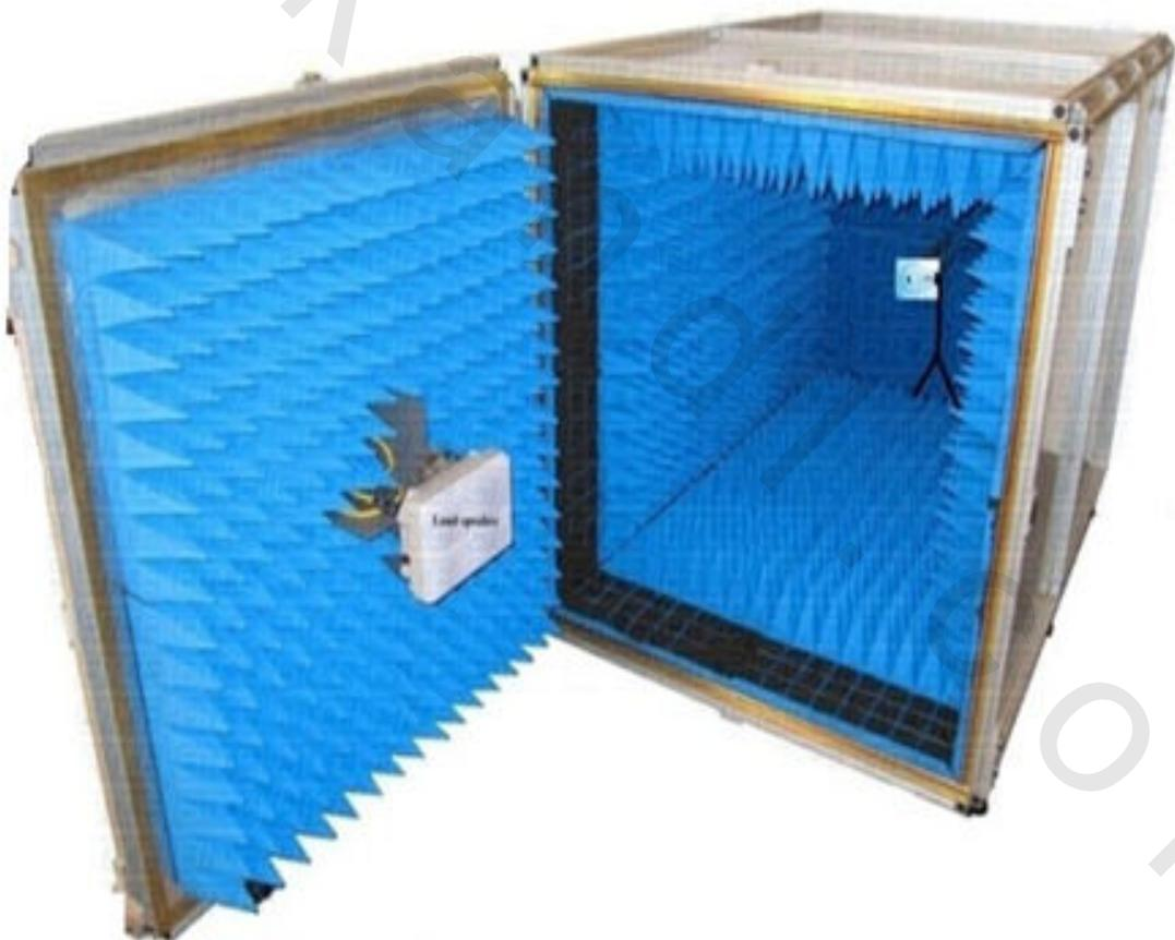
**Fig.(14):The anechoic chamber used for mice exposure to the MRI sound.**
