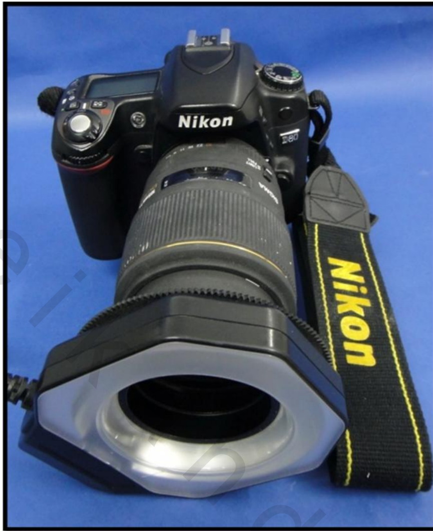
Figure 25: Digital camera supplied with a macro lens and a ring flash
