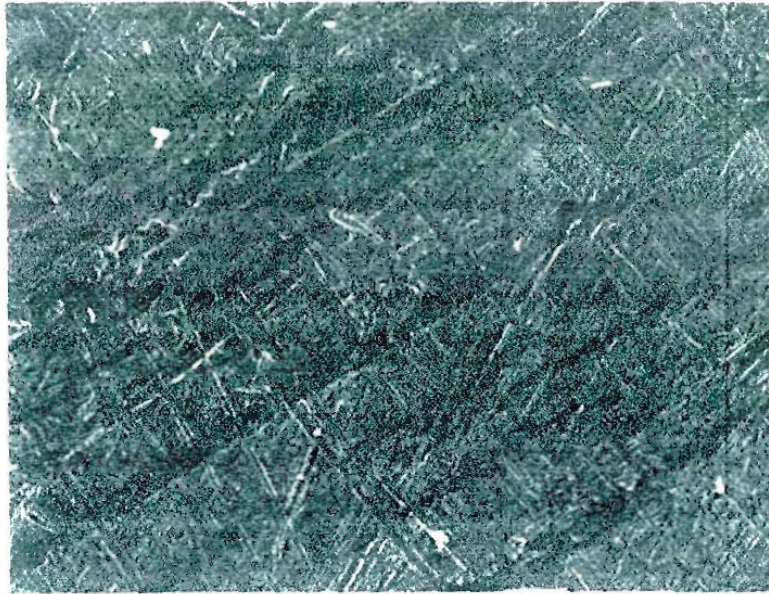
Fig. (4.50) SEM micrograph of carbon steel substrate, after removing the coating (magnification power 1000)
