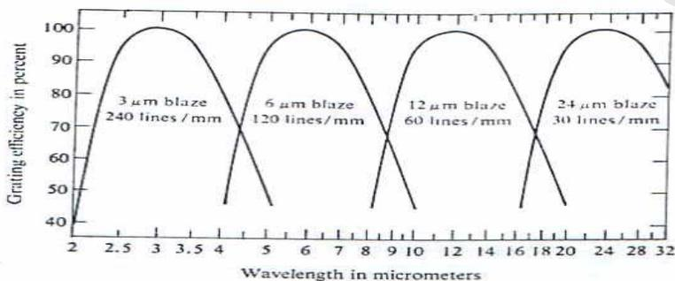
Fig. 3.10 Dispersion of infrared radiation by a diffraction grating.
