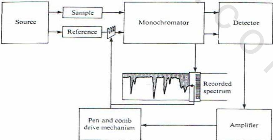
Fig. 3.1 Components of a typical double-beam infrared spectrophotometer.
