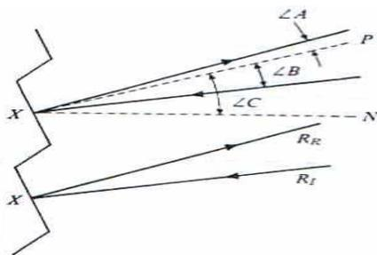
First-order diffraction of infrared radiation by a grating, where,  $\angle A$  is the angle between a perpendicular to the surface groove and the diffracted ray;  $\angle B$  is the angle between the normal line (perpendicular to the unblazed surface) and the incident ray;  $\angle C$  is the blaze angle. When  $\angle A = \angle B$ , the intensity of the diffracted ray will be at a maximum (maximum grating efficiency).
