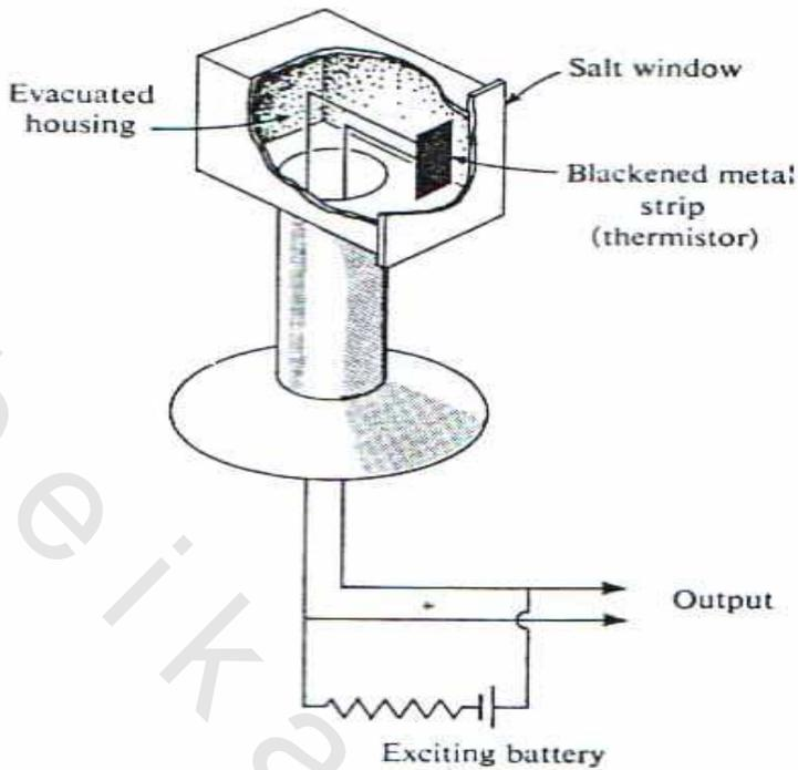
Fig. 3.6 Typical construction features of a bolometer detector.
