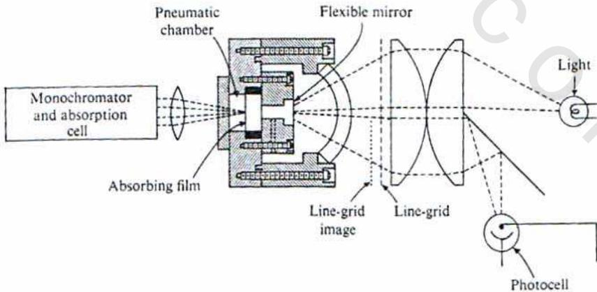
Fig. 3.8 Schematic diagram of a Golay detector.
