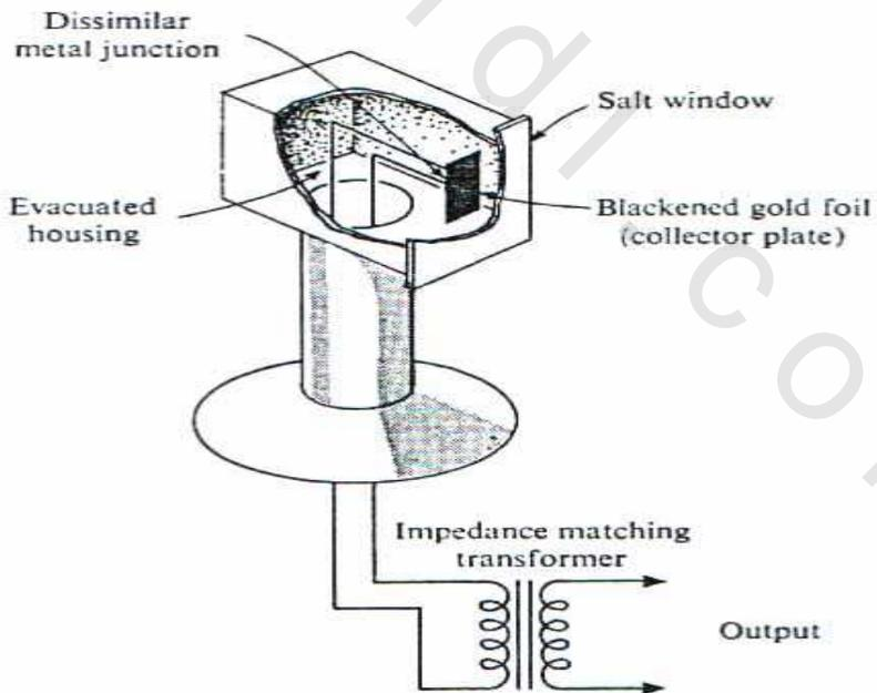
Fig. 3.7 Typical construction features of a thermocouple detector.
