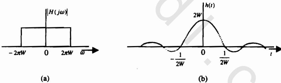
Fig. D.8. System function and impulse response of an ideal low-pass filter.
